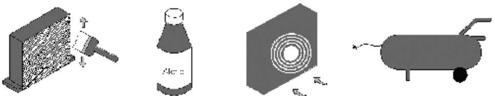
Figure 6 Cleaning of the Condenser
